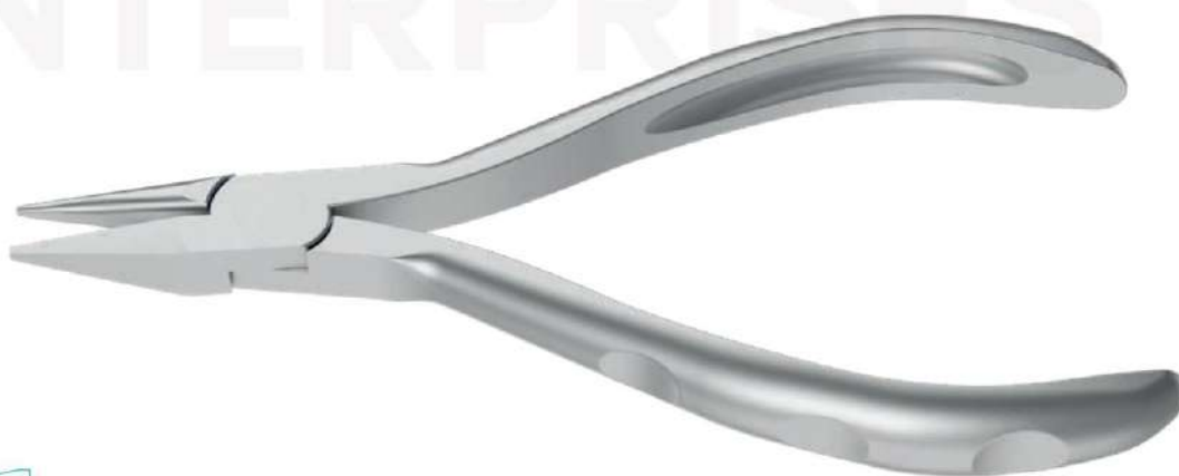
bird beak pliers ODE-1937 Light wire bird-beak pliers with a groove. The longer conical beak facilitates the creation of precise loops. The groove makes it easy to locate and duplicate loops. Wire size: max. 0.70 mm (0.028")
